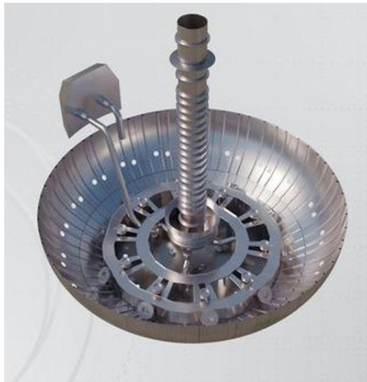
Fig. 2 – Render of oxygen tank lower part of SH7+ booster, version V1, with the lower section of central pipe for methane supply [8]
