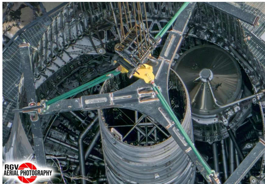
Fig. 5 – Lower part of SH18 booster, version V3, main oxygen tank with a side oxygen landing tank [9]
