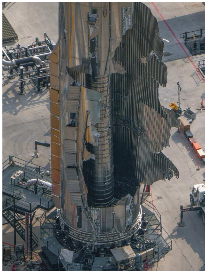
Fig. 1 – General view of internal components of SH18 (B18) booster – the first unit of new V3 version after unsuccessful cryogenic testing [7]
